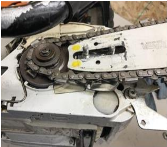
Chain installed on drive sprocket and aligning bar
