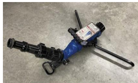
Shown here with smooth bore nozzle, a Blitzfire is a type of master stream device.
