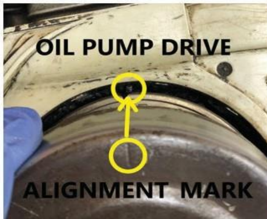
Aligning the clutch drum with the oil pump drive
