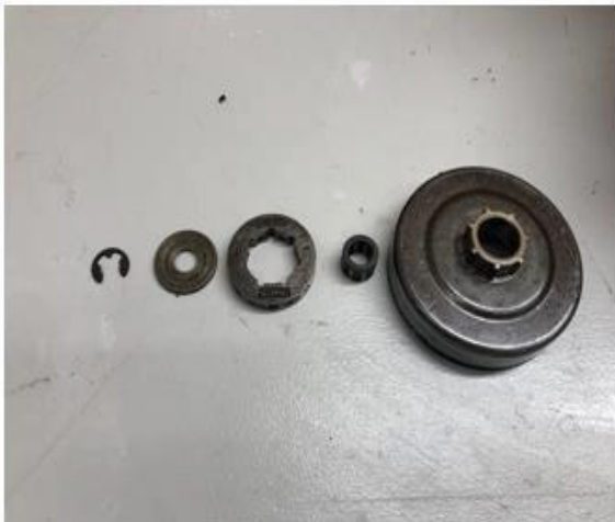
E-Clip, Washer, Sprocket, Needle Bearing, and Clutch Drum
